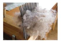
Release the comb and turn it 90° to the right. Comb with the other comb from top down. Turn the comb to the left and comb again.
