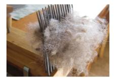
Comb the wool with the other comb. Start from one side. Change side and comb the wool from the other side. Make a swinging motion. Let the comb grab the top first and then go deeper and deeper.
