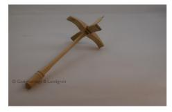
The shaft is inserted from the bottom into the wings. The holes shall fit together.
